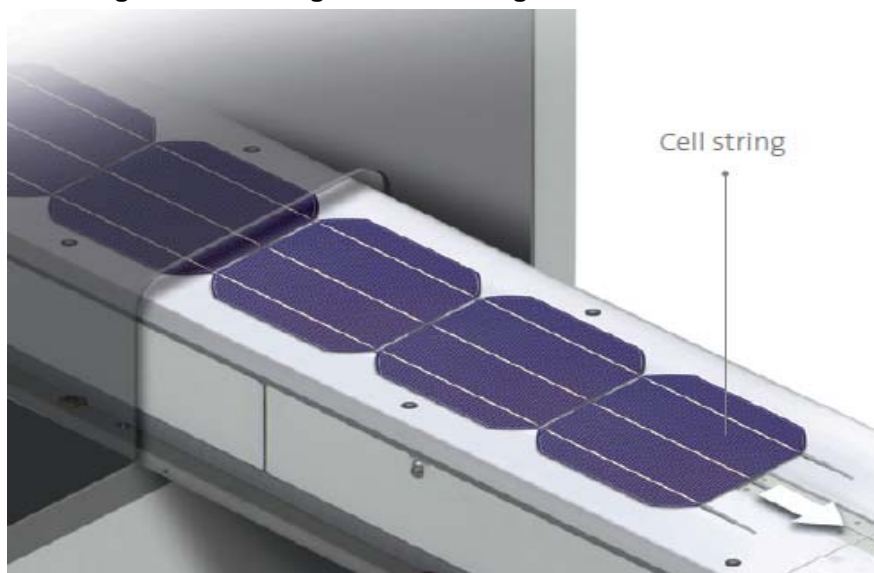
Figure I-12 Soldering CSPV cells together into strings
