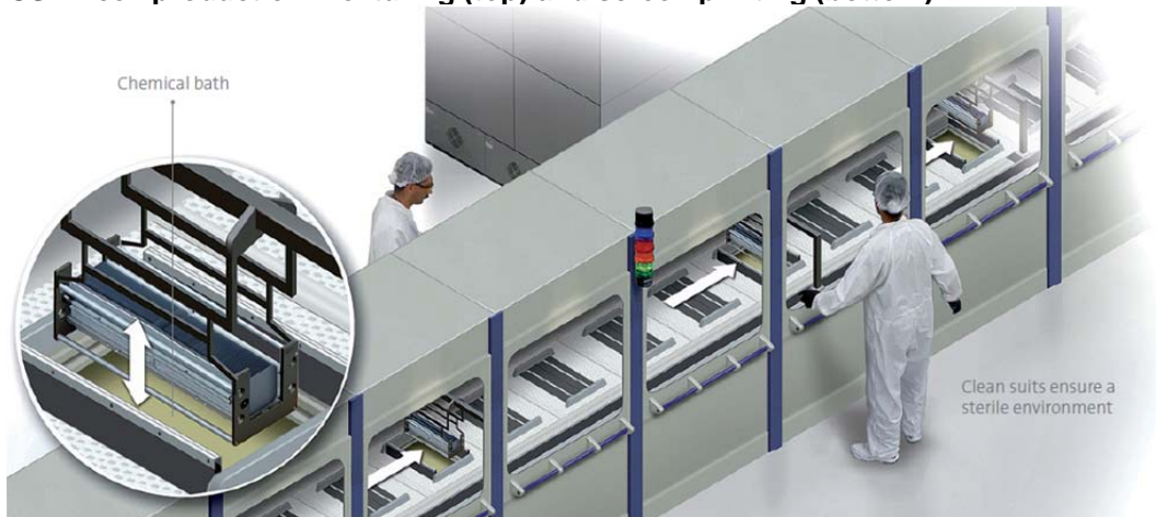
Figure I-11 CSPV cell production: Texturing (top) and screen printing (bottom)
