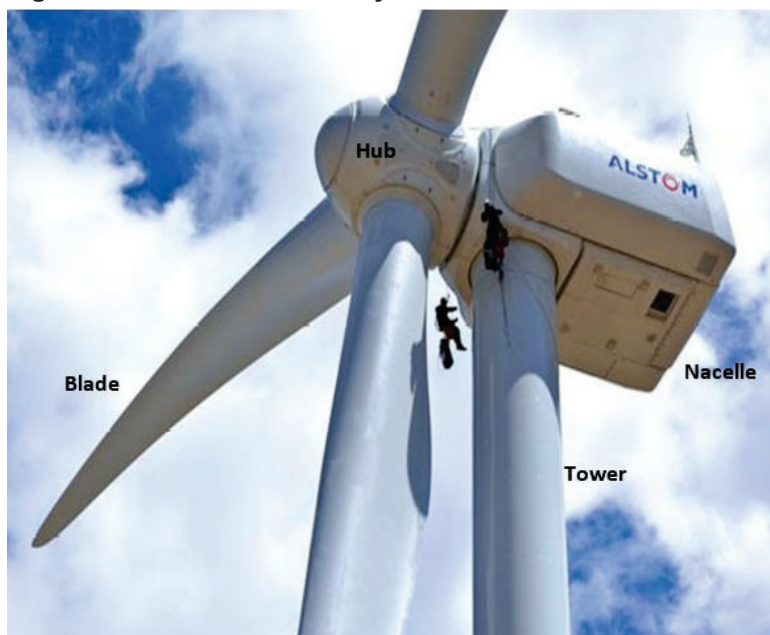
Figure 1.1 Wind towers: Utility-scale wind turbine
