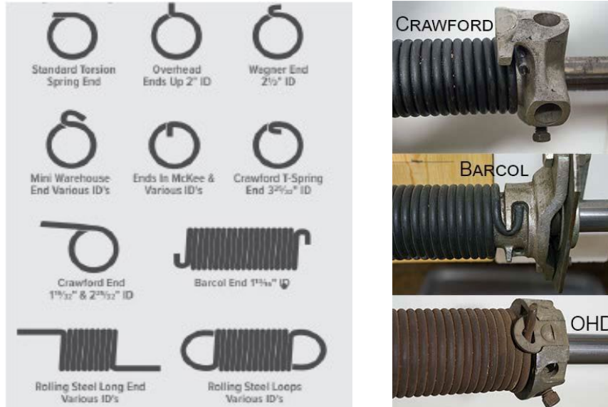
Figure 1.3 Overhead door springs: Other end shapes and fittings
