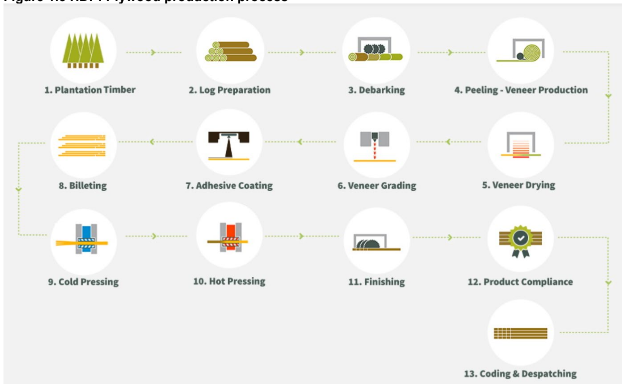
Figure 1.3 HDP: Plywood production process
