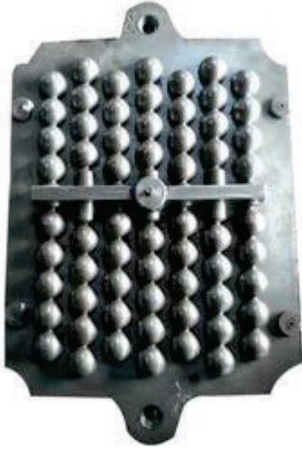
Figure 1.4 HCCIGM: Casting pattern for HCCIGM
