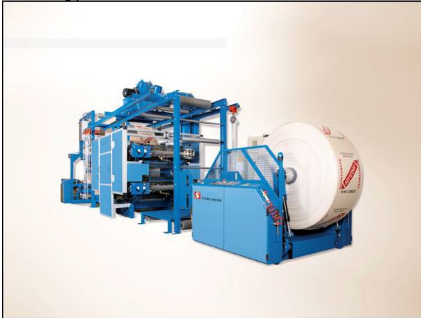
Figure I-4 LW sacks: Printing press
