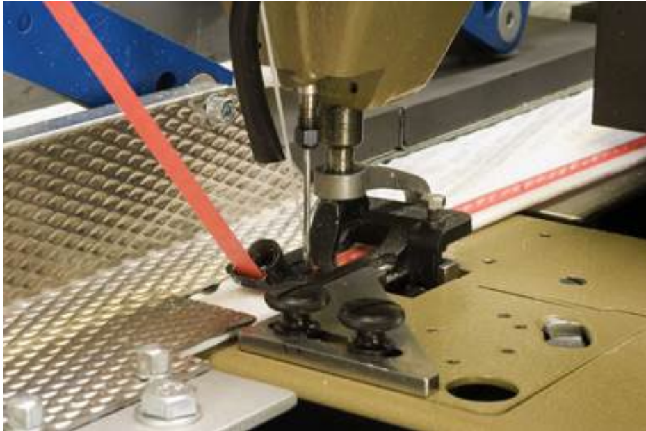
Figure I-7 LW sacks: Sewn end closure
