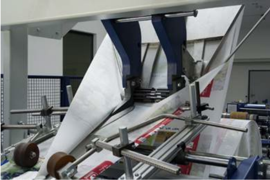
Figure I-6 LW sacks: Tubing process
