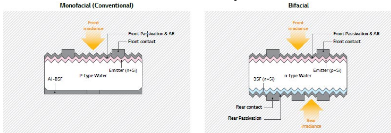
Figure I-3 CSPV cells and modules: Monofacial and bifacial cell design
