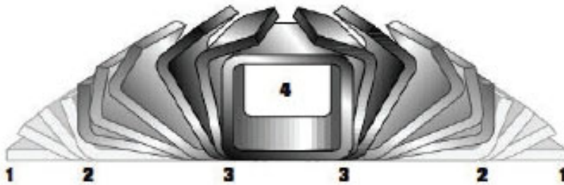
Figure I-2 Form-square weld-square process
