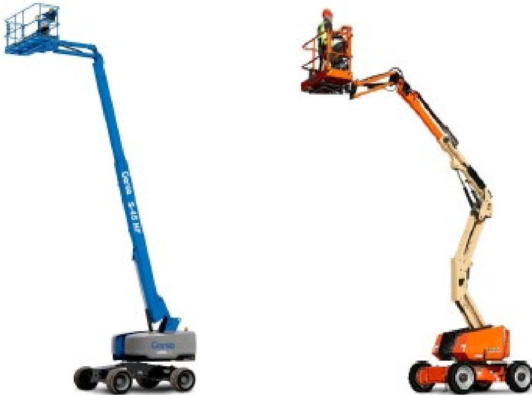
Figure I-3 MAE: Straight telescoping boom lift (left) vs articulating boom lift (right)
