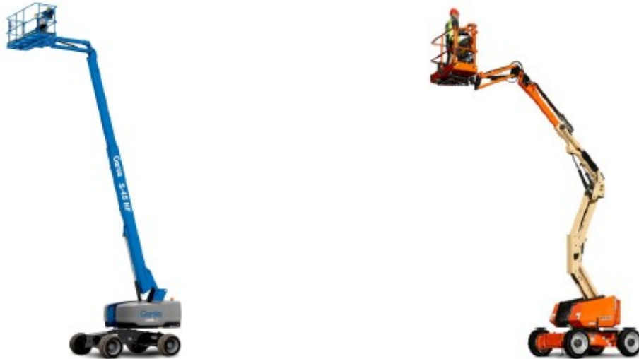
Figure I-3 MAE: Straight telescoping boom lift (left) vs articulating boom lift (right)
