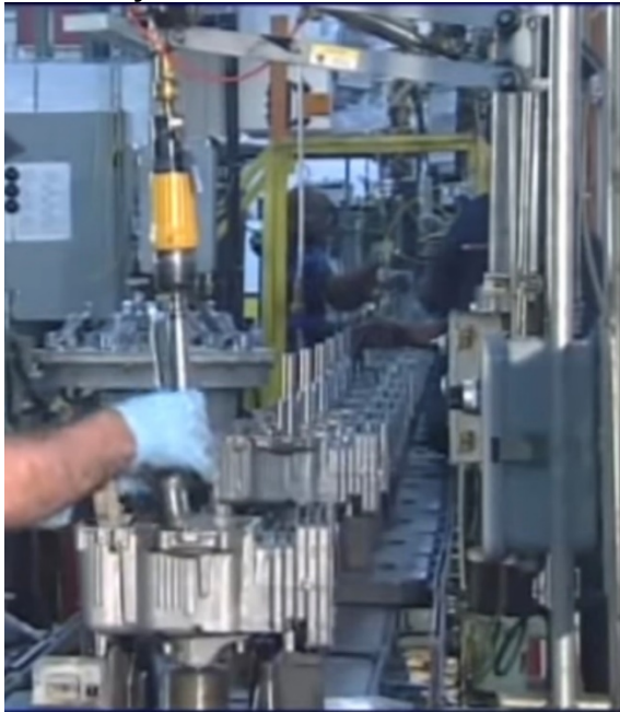
Figure I-5 SVSEs: Crank shaft assembly inserted into the cylinder box
