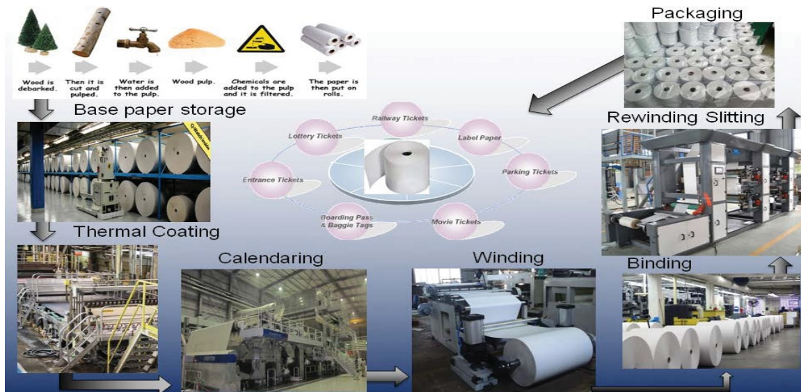
Figure I-1 LW thermal paper: Illustration of production process
