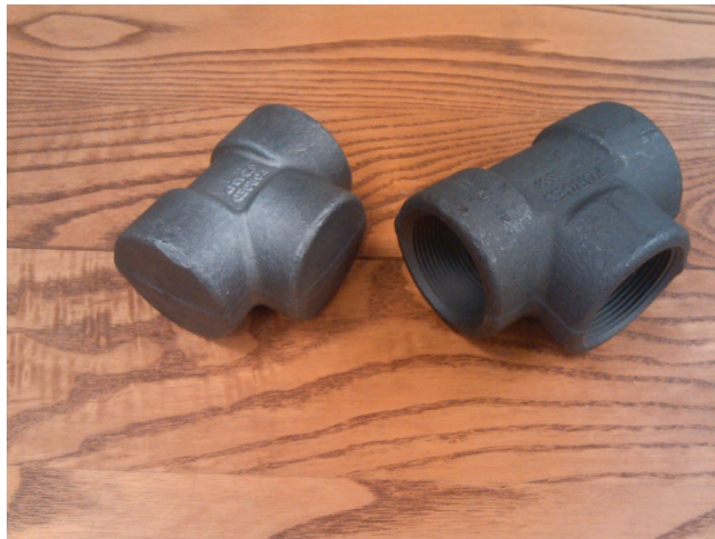
Figure I-6 FS fittings: Rough (unfinished) and finished
