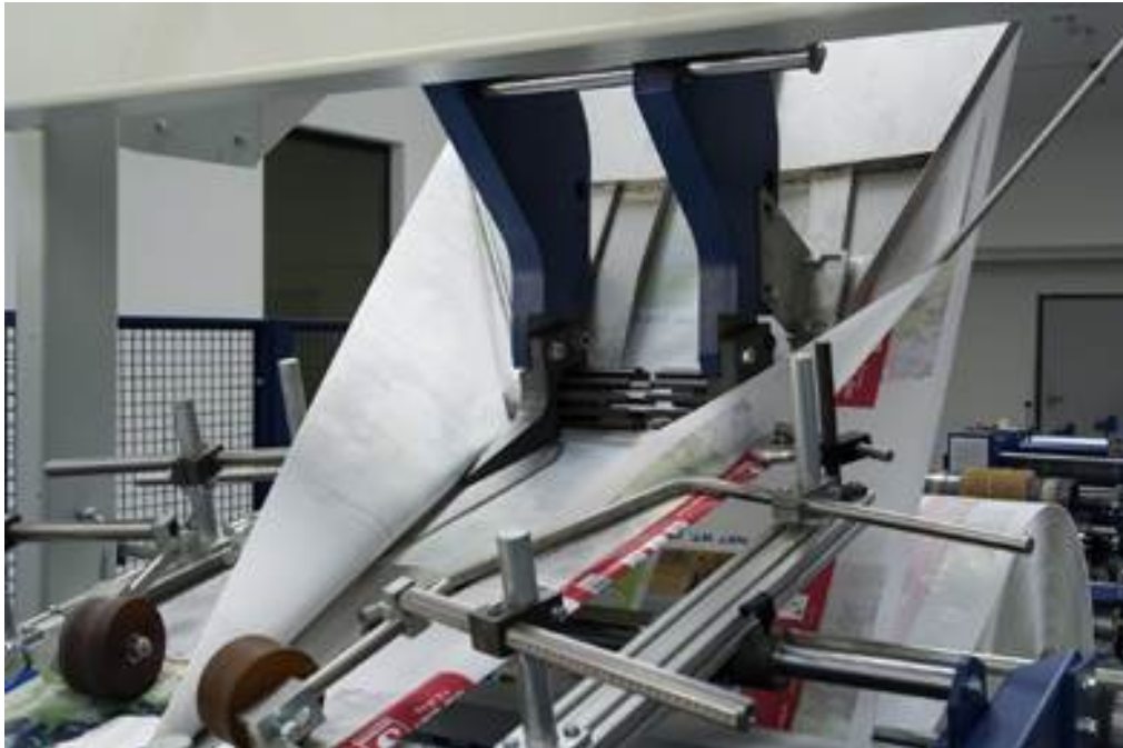
Figure I-5 LW sacks: Tubing process
