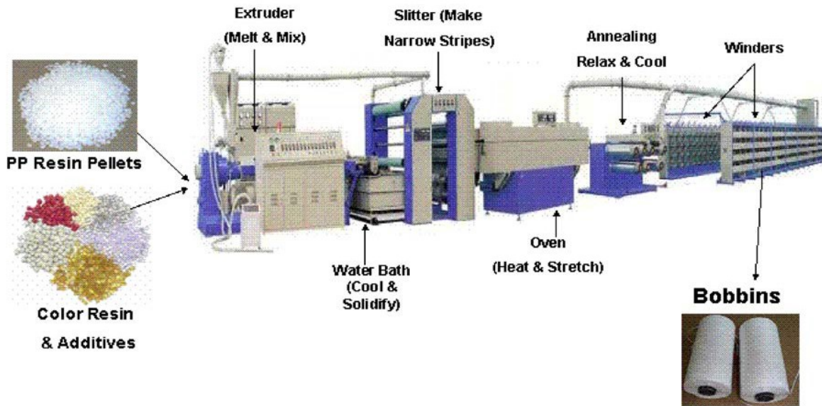
Figure I-1 LW sacks: Extrusion and slitter for producing polypropylene strips
