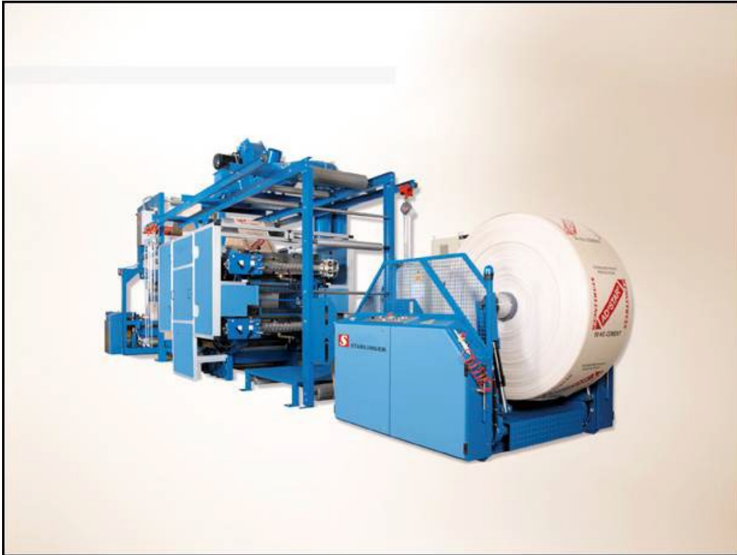
Figure I-3 LW sacks: Printing press
