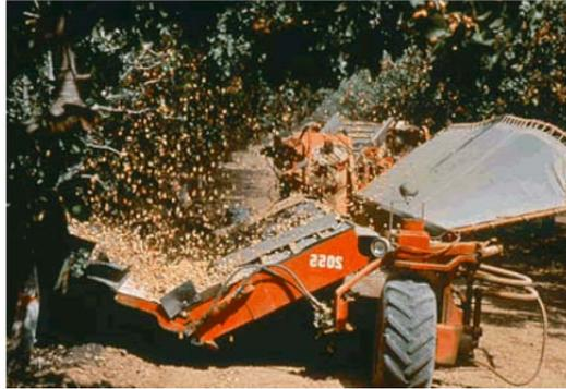
2. A mechanical harvester shaking tree
