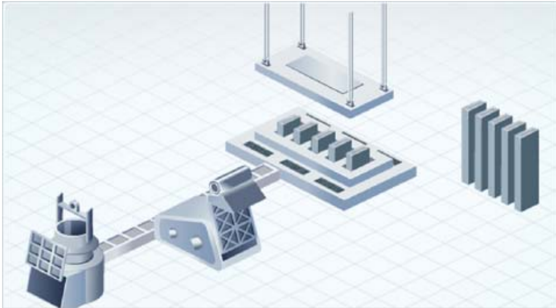
Figure I-4 Aluminum foil: Direct chill casting process
