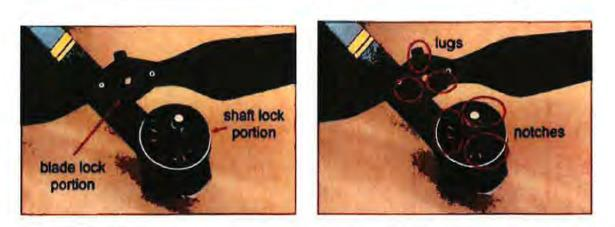
CDX.0001C.0048 (showing annotated version of a photo of the Mavic Pro marked as CX-0221); see also CX-0221. The lugs and notches of the Mavic Pro's locking mechanism can also be seen in the schematic of the Mavic Pro's rotor assembly. CX-0130. An annotated excerpt of the schematic is set forth below:
