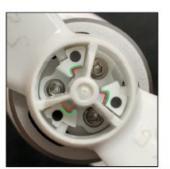
Figure 12. Lugs and Notches on the Phantom 4 (after engagement) (CPX-0021)
