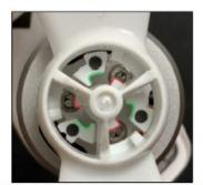
Figure 11. Lugs and Notches on the Phantom 4 (before engagement) (CPX-0021)
