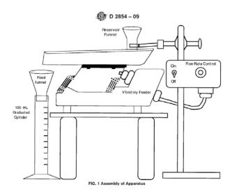
*Id.* at \*1-2. The test involves using the vibratory feeder to place granular adsorbent into the graduated cylinder to any preferred level (but to more than 50% cylinder capacity, and within certain mL/s speed range), and then weighing that amount in a "balance pan." *Id.* at \*2.
