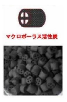
CX-0909C at Q/A 201; JX-0054C; RPX-0027. Each MPAC piece has a regular outside curved surface with a circular cross-section, bounded by two planar faces. This makes it at least "substantially cylindrical." Further, as determined above, the construction for "hollow cylinder"
