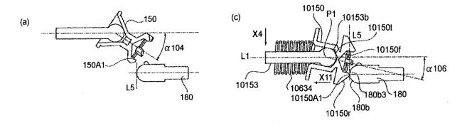
The coupling member shown in Figure 88(a) does not exhibit any axial movement, whereas the coupling member in Figure 88(c) combines pivoting with axial movement. As a result, coupling member 150 in Figure 88(a) requires a larger of angle of inclination ( $\alpha$  104) prior to engagement than is needed by coupling member 10150 in Figure 88(c) ( $\alpha$  106). *Id.*, col. 63:43-48.
