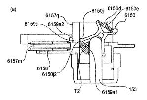
*Id.*, Fig. 65(a). So engaged, the locking member prevents the coupling member from pivoting from its inclined position. *Id.*, col. 53:19-24.
