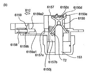
*Id.*, Fig. 68b. With locking member 6159 no longer projecting into the space of drum flange 6157, coupling member 6150 is able to pivot and come into alignment with drum shaft 153. *Id.*, col. 53:64-67. According to the specification, locking member 6159 is "movable" in the mounting direction X4 so that it can engage with drum flange 6157 and "moves" in the direction
