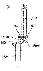
*Id.*, Fig. 22(b). As the process cartridge continues to move in direction X4 during the mounting operation, contact between the drive shaft and the upstream projection causes the coupling member to pivot until its axis (axis L2) is brought into alignment with those of the drive shaft (axis L3) and the photosensitive drum's shaft (axis L1). *Id.*, col. 27:15-39.
