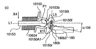
Id., Fig. 88(c). Compressing urging member 10634, coupling member moves in direction X11, so that the coupling member moves towards the tip of drum shaft 10153 closing the gap between coupling member 10150 and drum shaft 10153. *Id.*, col. 63:22-30. At the same time, coupling 10150 rotates so that it is inclined downstream. *Id.* With the coupling member so positioned, downstream projection 10150A1 of coupling member 10150 passes by the end of drive shaft
