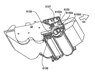
*Id.*, Fig. 63. In order to lock the coupling member in an inclined position when the process cartridge is not mounted in the printer, spring member 6158 pushes locking member 6159 against drum flange member 6157. *Id.*, col. 53:15-18. Pressed against drum flange member 6157, locking member 6159 engages with an opening in drum flange member 6157 so that a portion 6159a1 of locking member 6159 projects into space portion 6157b of the drum flange member 6157. *Id.*, col. 52:59-53:19.
