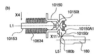
Pushing coupling member 10150 towards drive shaft 180 leaves a gap between coupling member 10150 and drum shaft 153 (highlighted). As the process cartridge is pushed in direction X4 during the mounting process, contact between driveshaft 180 and downstream projection 10150A1 of the coupling member results in the coupling member moving in two directions.
