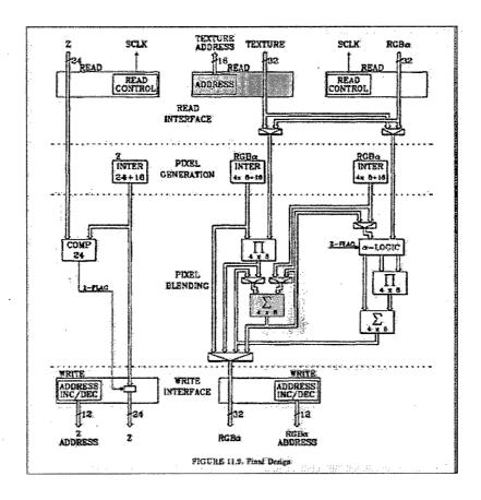
(RDX-367.) According to Respondents, the above figure shows the claimed texture look-up module in purple, shading module under NVIDIA's infringement theory in orange, and the feedback loop in green. (*Id.*) Respondents' expert, Dr. Crawfis, testified in detail that under
