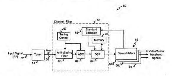
JX-0001 at Fig. 2. The digital processing in the channel filter allows for compatibility with multiple different television standards without using the multiple channel filters required in the prior art. *Id.* at 4:12-16. A bank of demodulators generates video and audio baseband signals, which can be decoded for playback on a view screen. *Id.* at 5:43-52. Claim 1 of the '585 patent reads:
