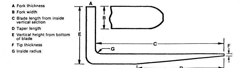
sizes--all of the dimensions listed in figure 1 (the cross section, blade length, tip thickness, blade height, taper length, etc.) may be individually specified--although there are certain standard sizes of forks (see below). Only 10 to 20 particular sizes account for the majority of fork arm sales.
