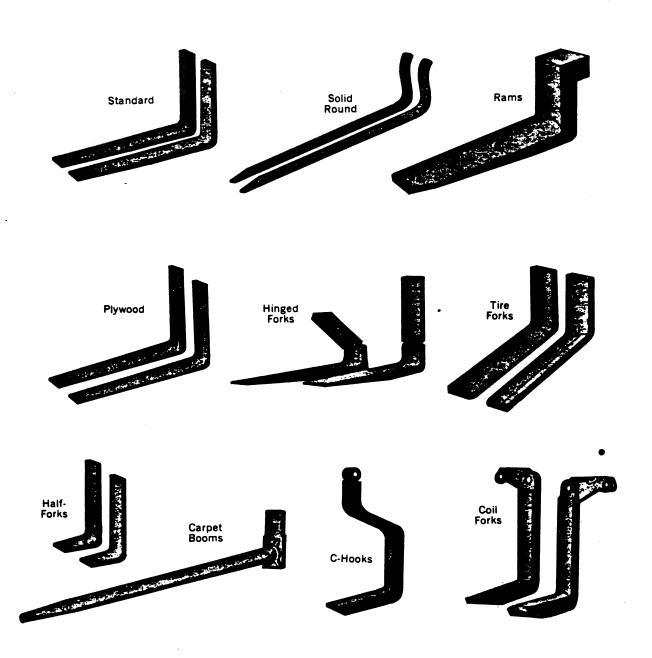
Figure 3.—Hook-mounted and shaft-mounted steel fork arms.
