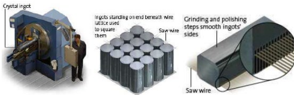
Figure 1.12 Wafer production: Cutting off the top and tail (left), squaring (middle), and slicing into wafers (right)
