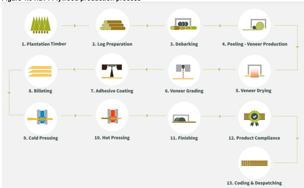
Figure 1.3 HDP: Plywood production process
