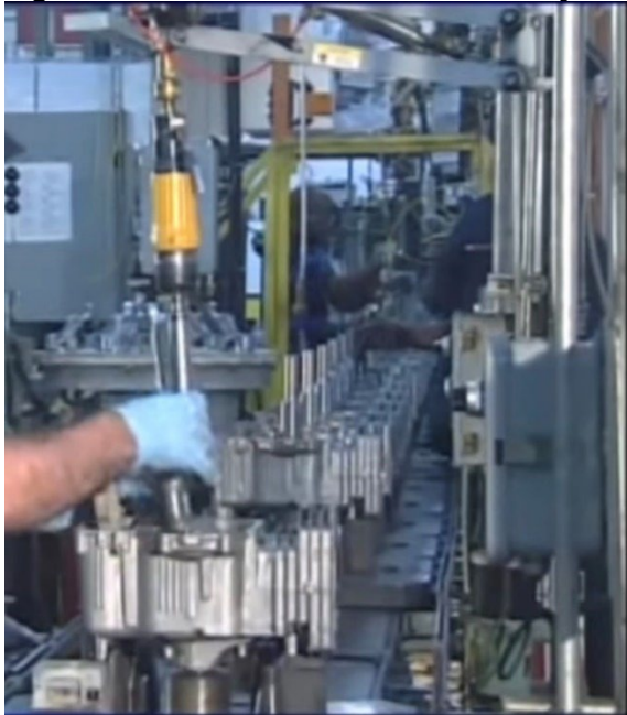
Figure 1.5: LVSEs: Crank shaft assembly inserted into the cylinder box
