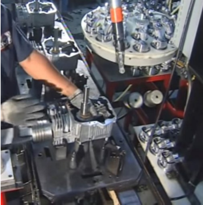
Figure 1.6: LVSEs: Piston installed into the cylinder
