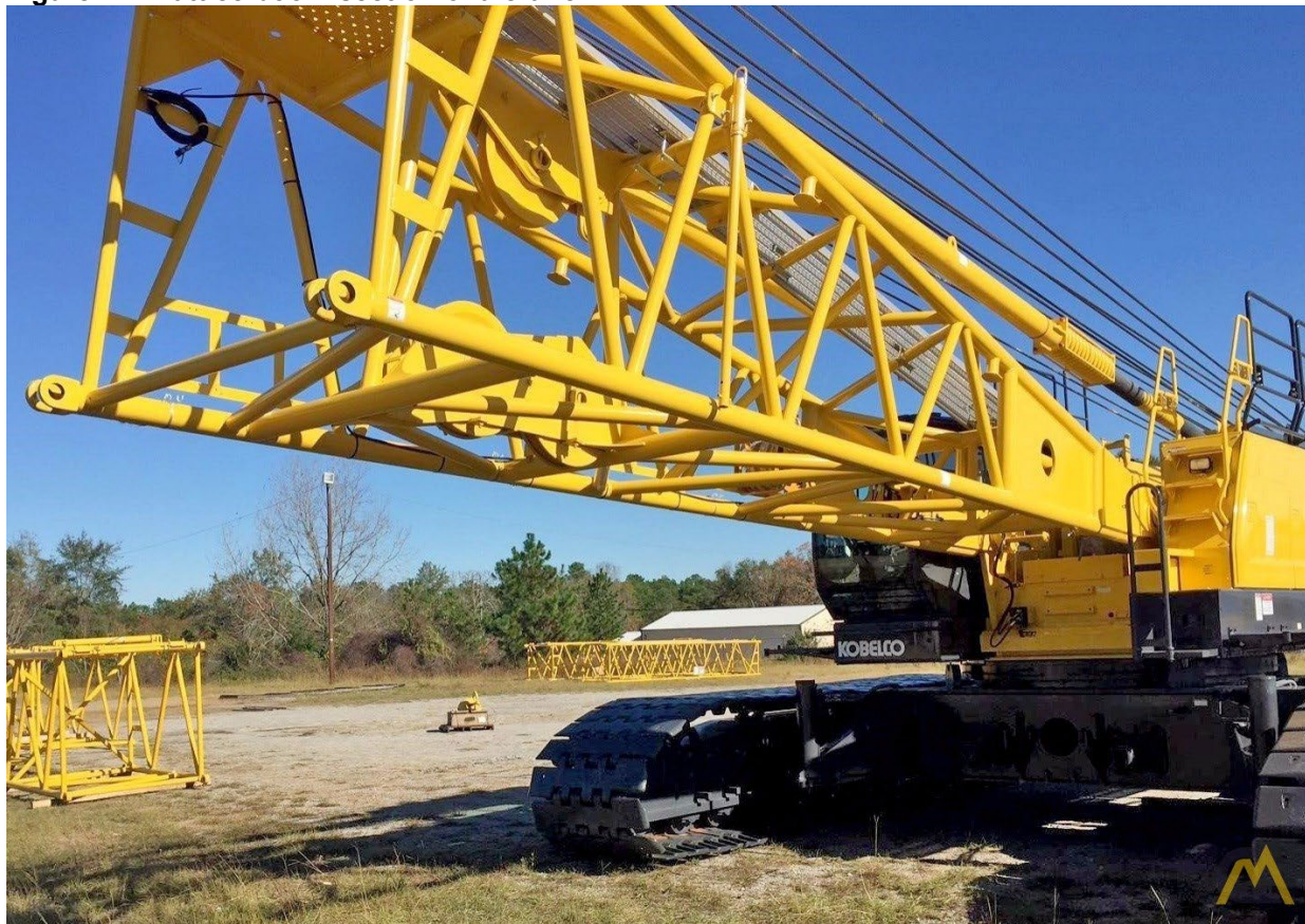
Figure 1.4. Lattice boom section of a crane
