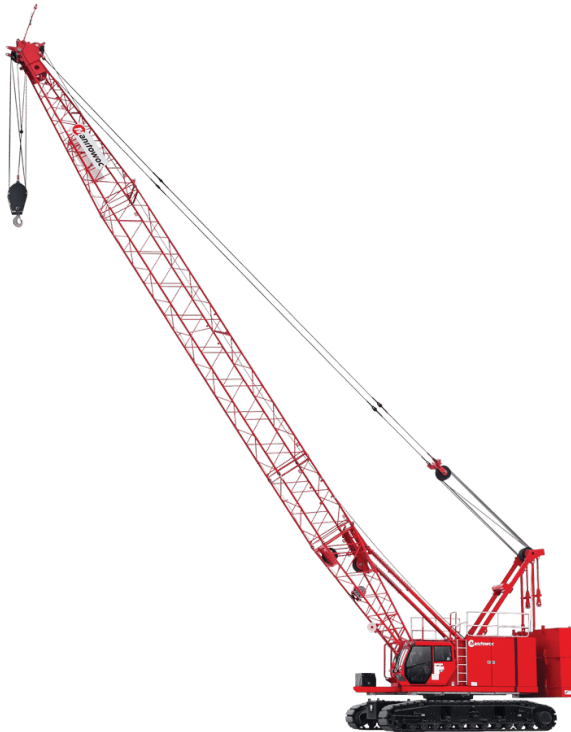
Figure 1.2. Lattice boom crawler crane
