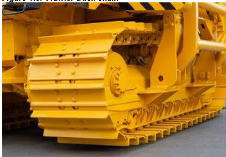
Figure 1.3. Crawler track chain
