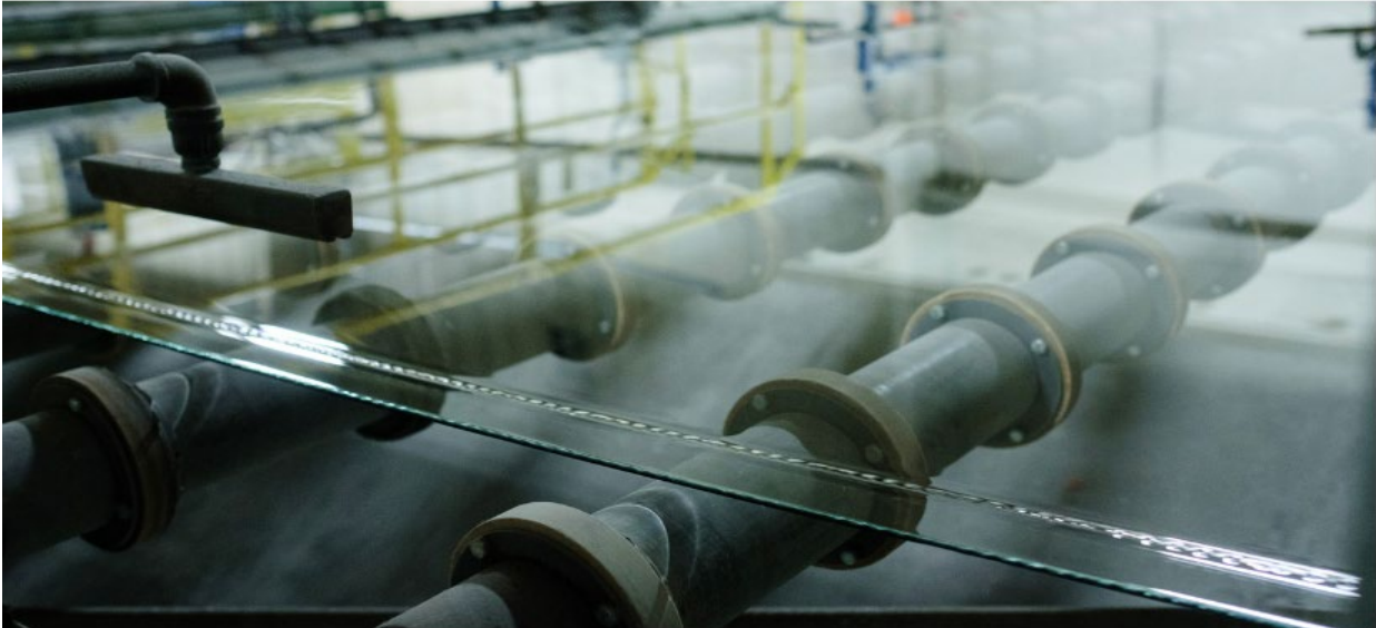
Figure 1.1 FGP: Float glass ready for inspection and cutting
