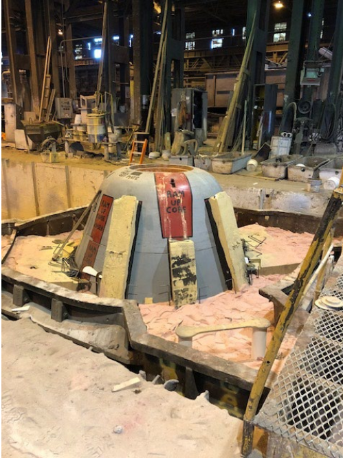
Figure 1.3. Slag pots: Molding process
