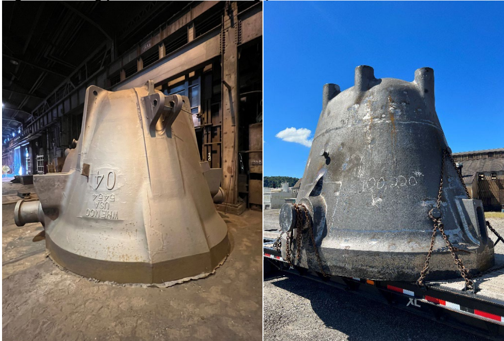
Figure 1.1. Slag pots: Finished cast slag pots
