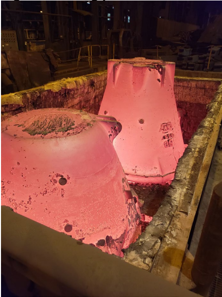
Figure 1.5. Slag pots: Heat treatment
