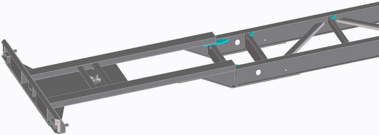
Figure 1.10 Gooseneck combined with main frame
