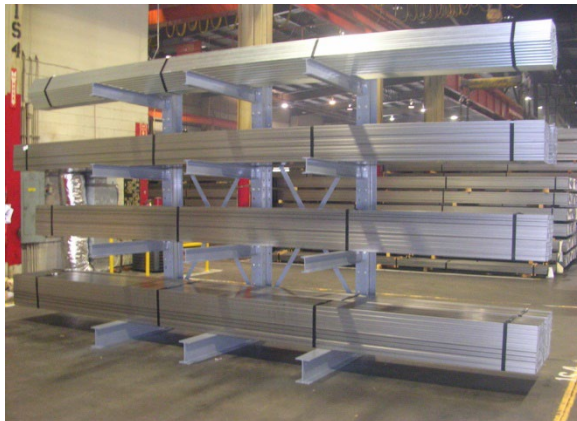
(I-2b) Cantilever rack configuration
