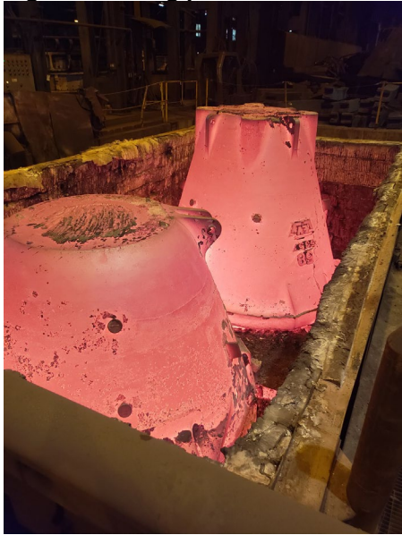
Figure 1.5. Slag pots: Heat treatment
