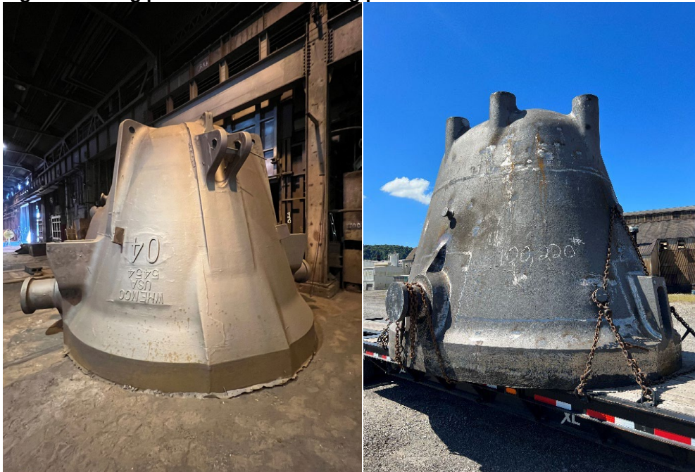
Figure 1.1. Slag pots: Finished cast slag pots
