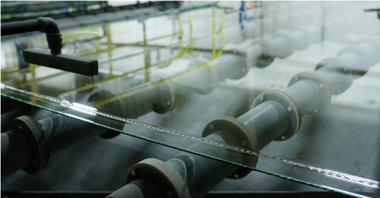
Figure 1.1 FGP: Float glass ready for inspection and cutting
