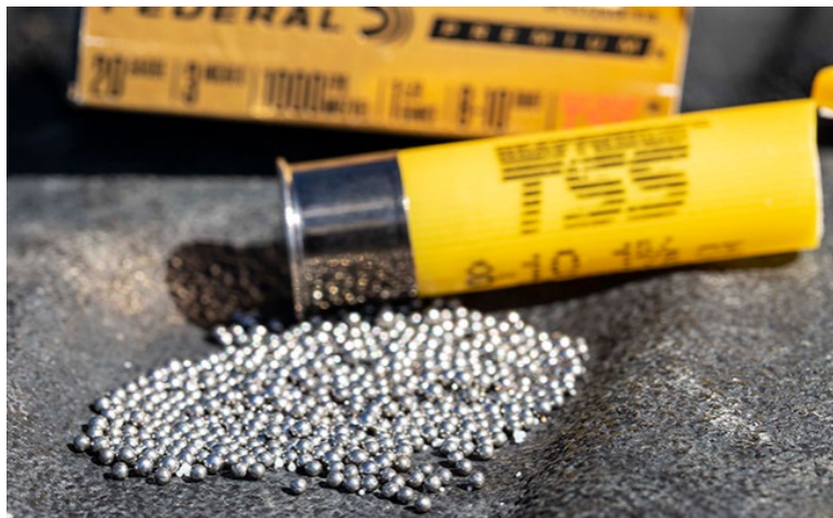
Figure I-2 Tungsten shot: Tungsten super shot (“TSS”) shotgun shell and individual tungsten shot pellets
