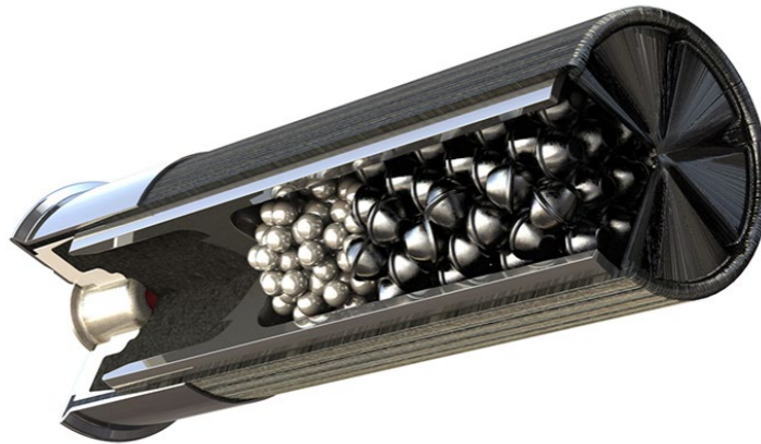
Figure I-1 Tungsten shot: Cut-away view of a shotgun shell showing the individual tungsten shot pellets
