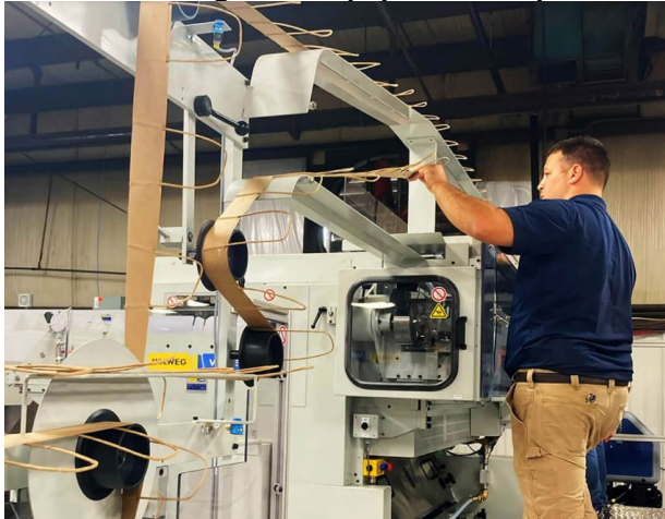
Figure I-9. Machine making twisted paper handle patches
