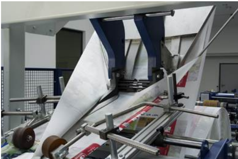
Figure I-6 LW sacks: Tubing process
