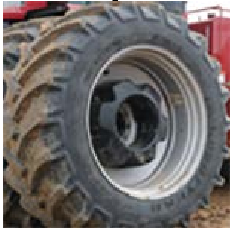
Figure I-8 OTR tires: OTR agricultural wheel and tire assembly
