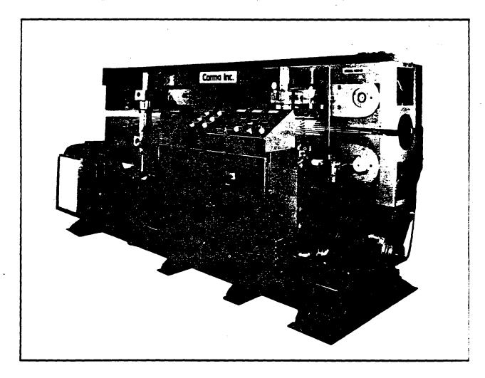
The model 420 corrugator is mounted on two base plates in which height and sideways adjustments are incorporated.
