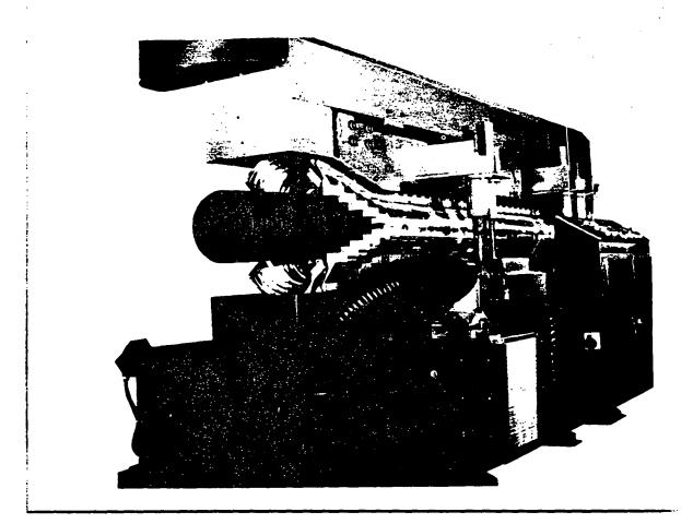
The model 3020 corrugator is able to produce a wide range of pipe sizes. To do so, a manually operated variable centre height adjustment has been incorporated. This feature enables one to maintain the centre height of the corrugator for all moldblock sizes.
