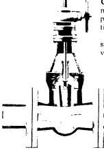
Gate valves, in carbon, alloy and stainless steel, stop or permit flow by moving a wedge-shaped metal gate in or out of the line of flow. Gate valves perform extremely well in high temperature and high pressure applications and corrosive environments.
