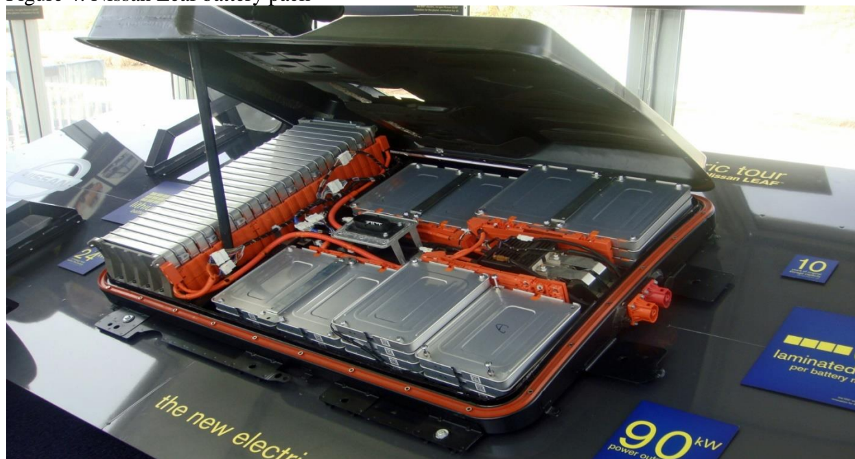
Figure 4: Nissan Leaf battery pack
