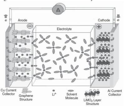
Figure 3: The structure of a lithium-ion battery cell
