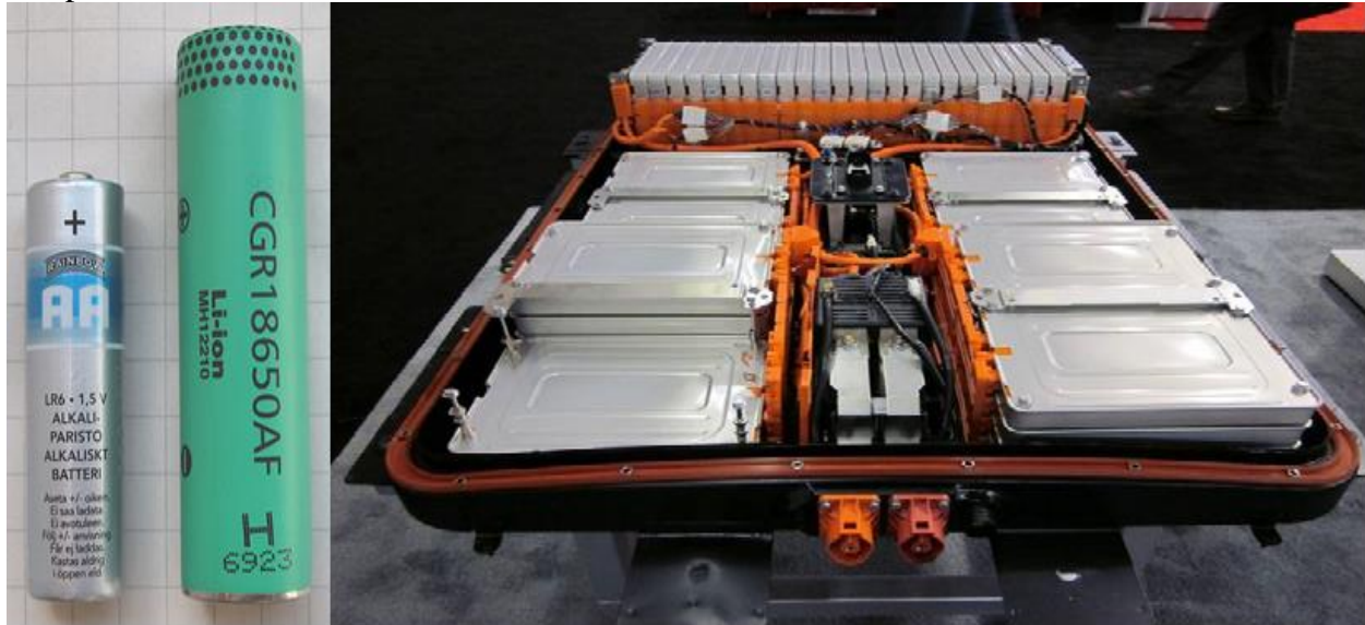
Figure 2: Alkaline AA battery cell, Tesla lithium-ion battery cell, and Nissan battery modules and pack
