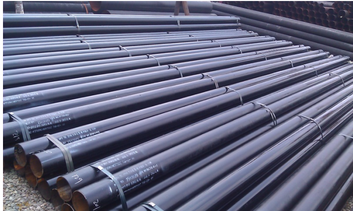
Figure I-1: Welded API line pipe
