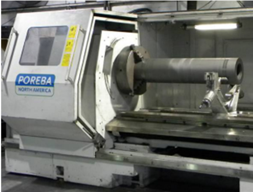
Figure 1.4 Machining the outside surface of a graphite electrode
