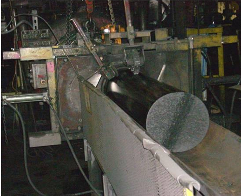
Figure 1.3 A graphite electrode form being extruded
