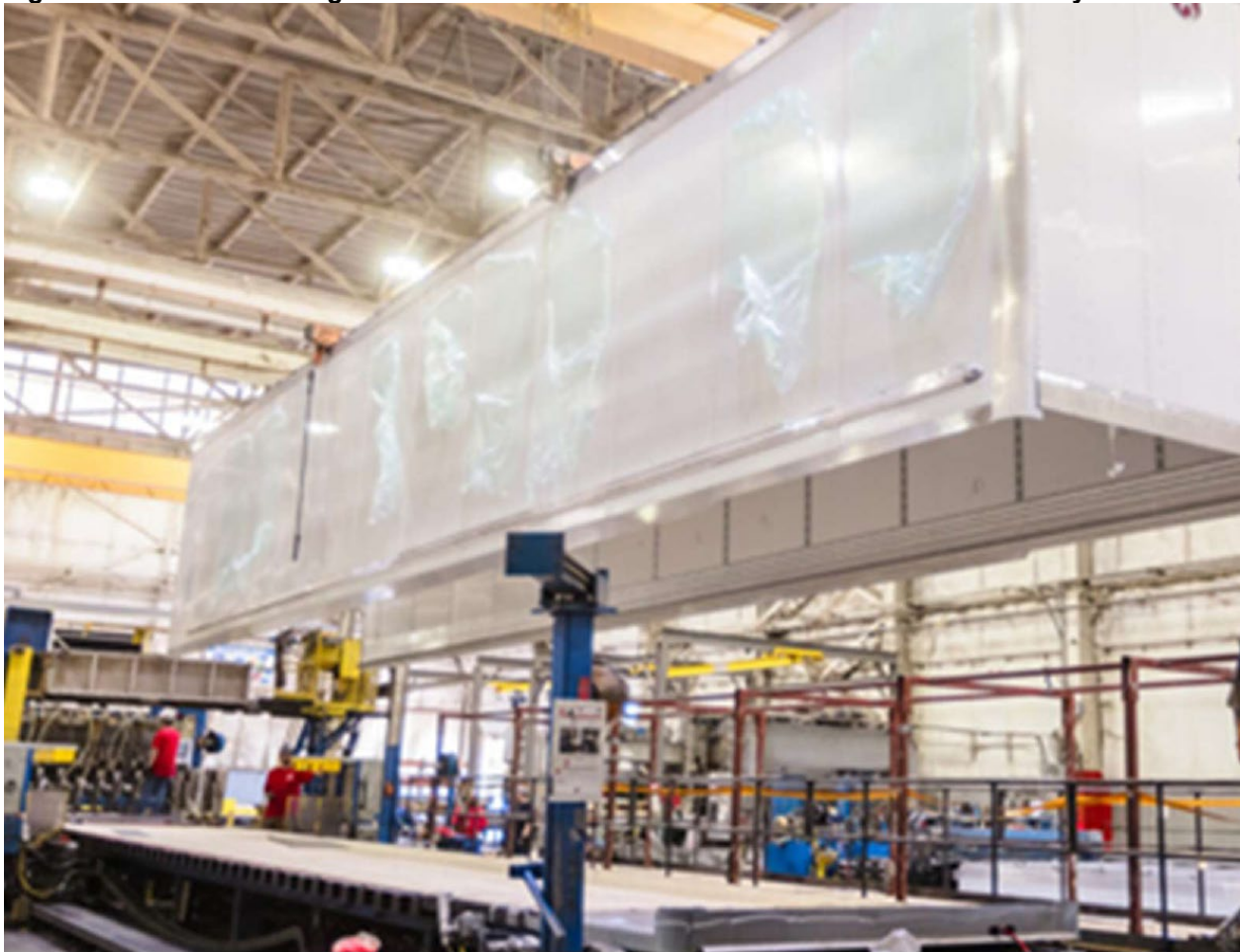
Figure 1.5: A crane moving a “box” onto the subframe and floor on the main assembly line
