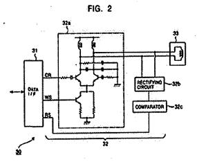
According to the '596 patent, the remote memory chip 4 of a tape cassette "can transmit data by performing adio communication with a remote memory interface 30 of FIG. 1, in a tape streamer drive using an antenna 5." *Id.* at 4:17-20. Specifically, when a tape cassette is loaded into the "tape strea are drive, 10 of FIG. 1," "the remote memory chip is set to be in condition
