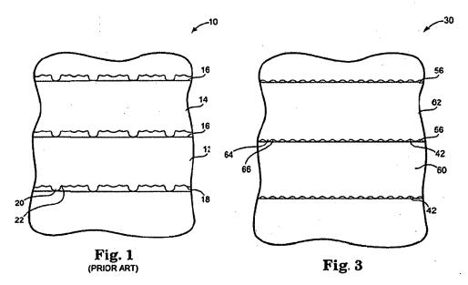
Specifically, as shown in Figure 3, the backside of the invention has a large number of peaks with relativel *i* small and uniform heights so that a "relative y large plurality of peaks 64 contact[:] the recor ling surface 56 of an adjacent winding 60 or 62." *Id.* at 5:52-55. These
